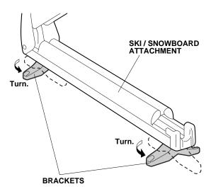
4. Using the supplied wrench, install the ski/snowboard attachment to the front crossbar with four bolts, four collars, and two brackets.
