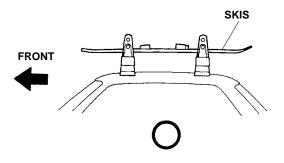
If the bindings cannot be positioned between the front and the rear attachments, install the skis with the rear bindings behind the rear attachment as shown.
